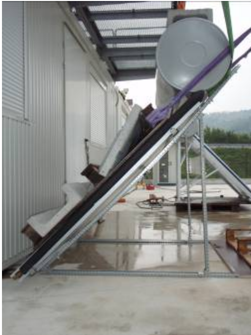
Figure 5 Example of a separable system mechanical load test with “stone load”.
