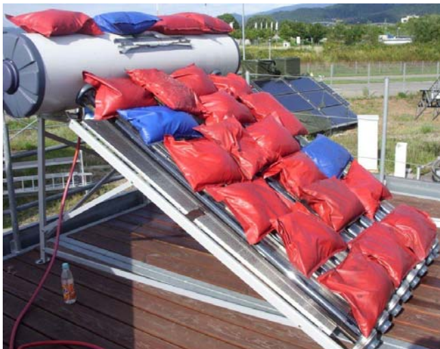
Figure 4: Example of a non separable system, mechanical load test with sand sack
