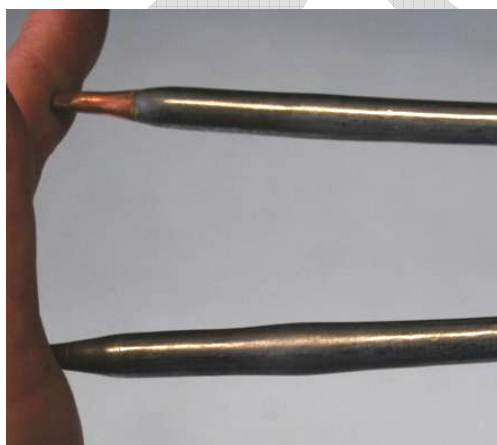
Fig. 15: Comparison of assembled and single heat pipe after 20 test cycles.
