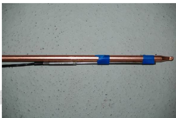
Fig. 08: Reference temperature sensor
