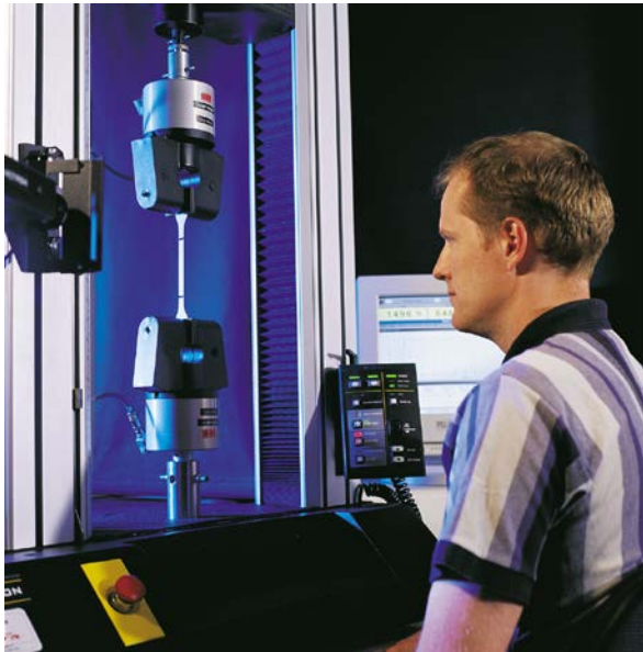
Figure 3. Tensile tester used for determination of maximum elongation and tensile strength
