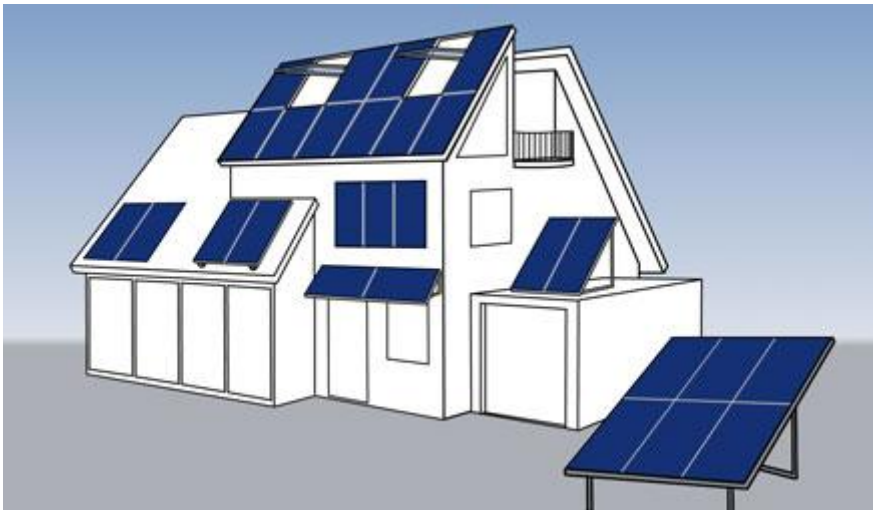
Figure 4: Illustration of different mounting situations
