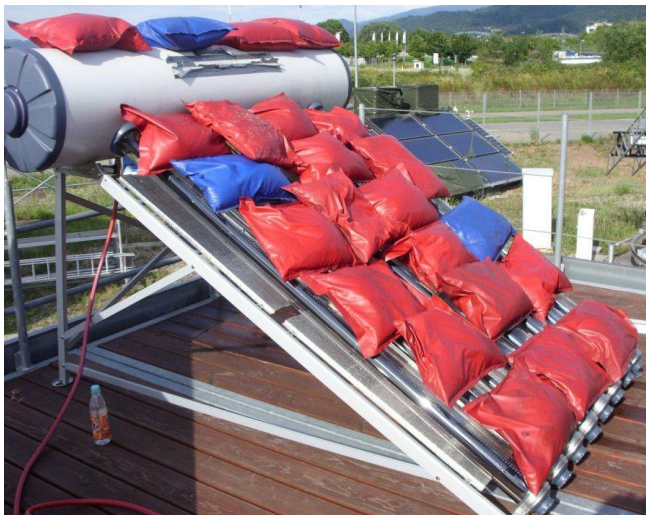
Figure 8: Example of a non separable system, mechanical load test with sand sack
