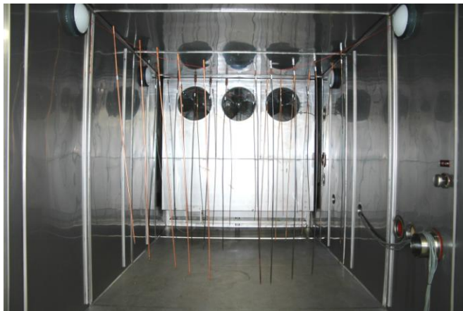
Figure 1: Climate chamber for temperature cycling test in SEACC laboratory
