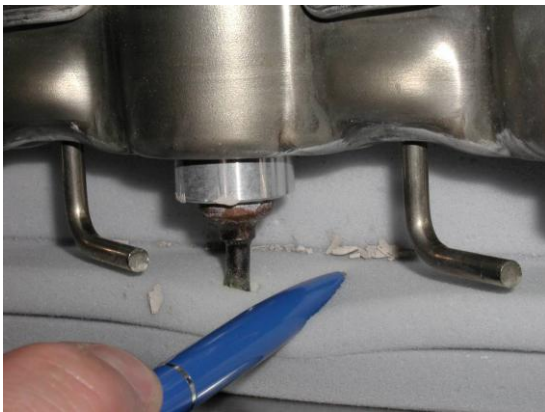
Picture 33) Fragments of heat transfer paste in manifold casing (after 30 days exposure)
