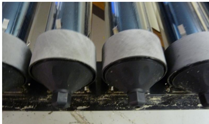
Figure 27: discoloration of vacuum tubes gaskets
