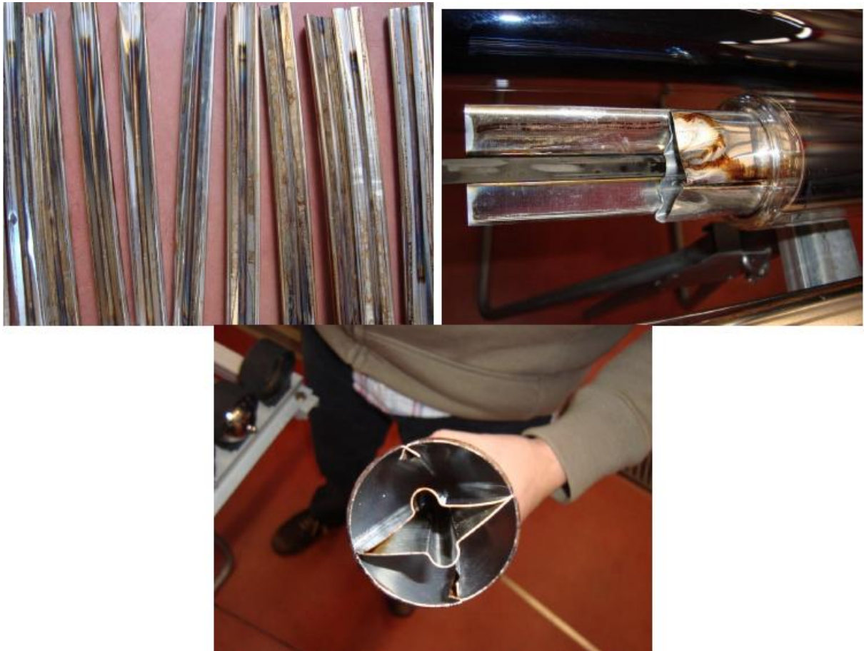
Figure 9,10,11 : Problems observed with the collector fins
