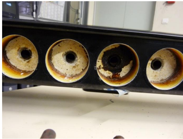
Figure 26: view of cracked gasket
