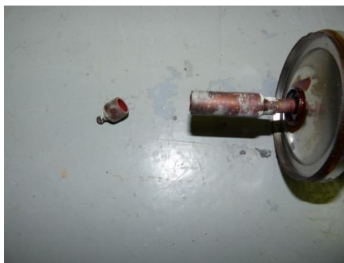
Figure 25: view of heat pipe opened
