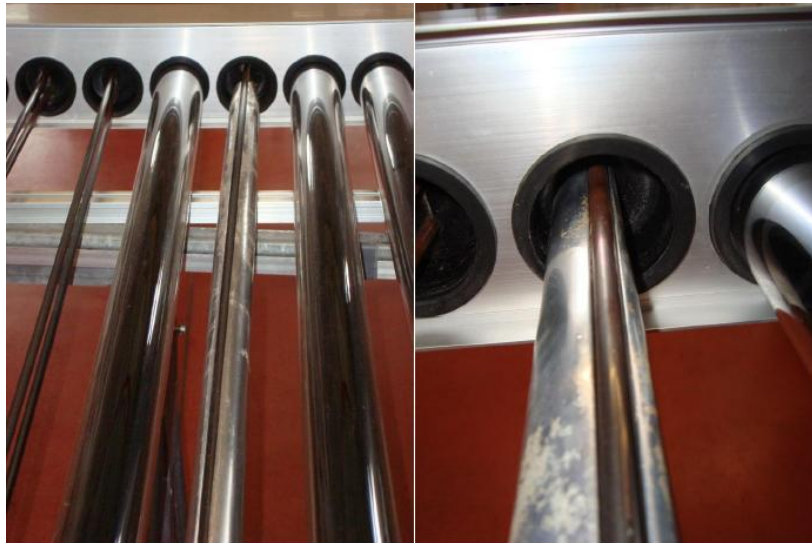
Figure 2,3: Fins deformed with some points having poor contact with the absorber
