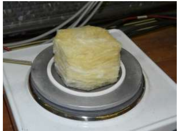
Figure 3: Test sample placed on the aluminium disc. The black fleece is placed on the heating plate to simulate direct contact with a hot absorber.
