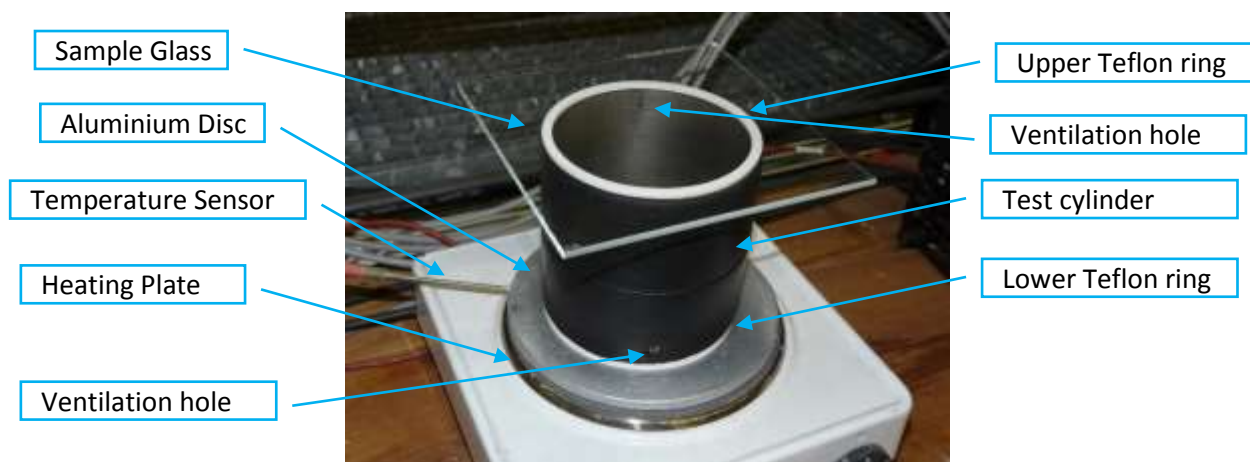
Figure 1: Test device for laboratory testing of outgassing
