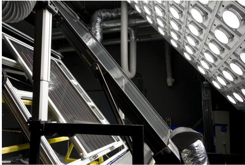
Figure 27. IAM measurement in solar simulators requires more parallel light than the standard efficiency tests.
