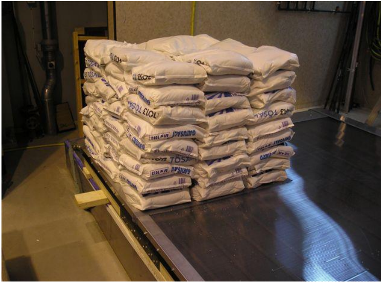
Figure 4. Positive mechanical load on collector cover. Beware that un-even distribution of load, as in this example, may cause unrealistically high stress
