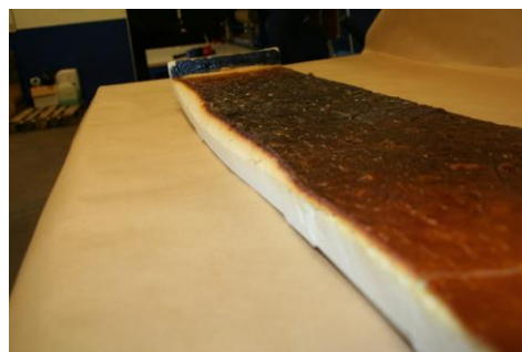
Figure 25 Degradation of insulation
