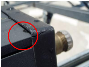
Figure 11 Cracking of polymeric parts of manifold
