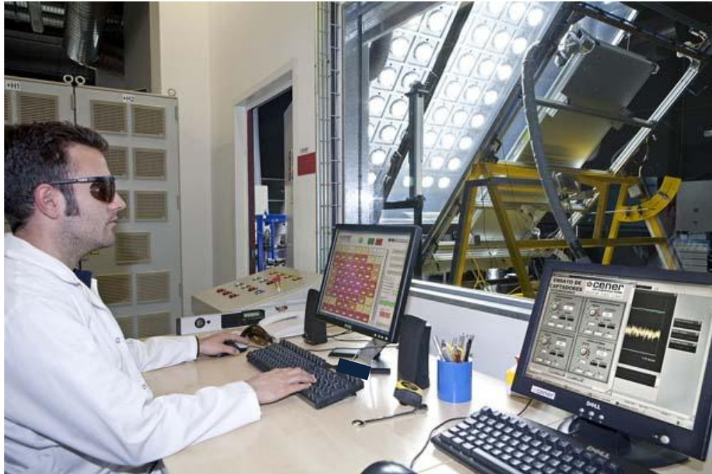
Figure 26. Performance testing in solar simulator
