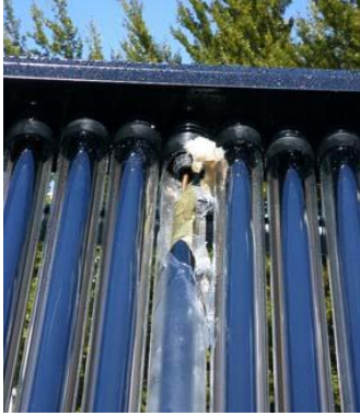
Figure 15 Cracked glass after external thermal shock test
