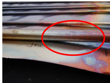
Figure 19 Loss of bonding absorber tubes
