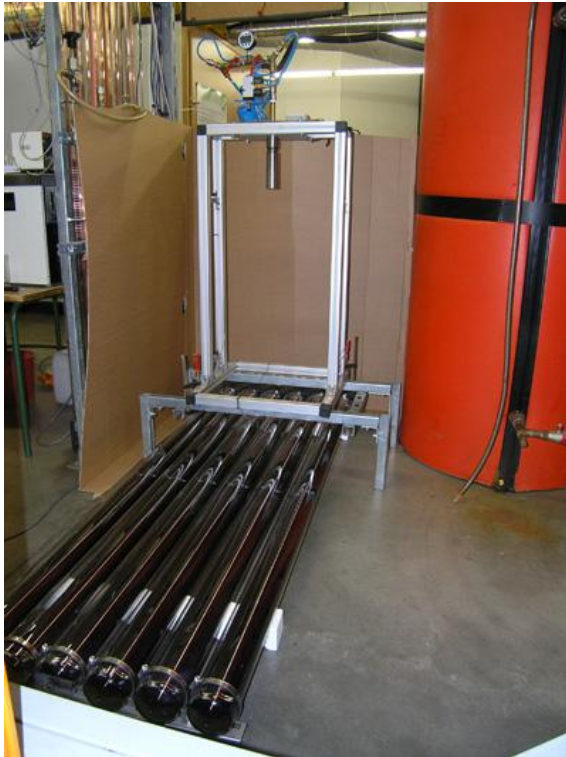
Figure 8. Ice ball launcher for vertical shots on collectors (using a loading device for single ice balls, adjustable pressured air and photo sensors)
