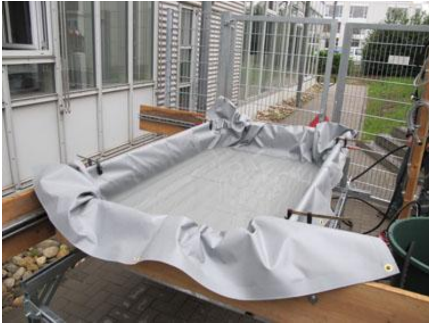
Figure 6. Simple setup for positive load test on evacuated tube collectors (using an adjustable wooden frame, a tarpaulin and water)
