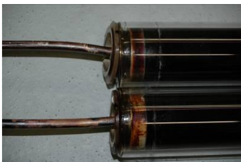
Figure 24 Outgassing within Vacuum Tubes
