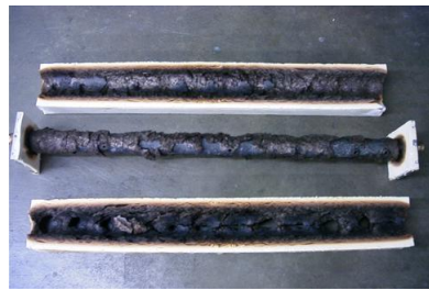
Figure 22 Degradation of PU foam insulation in manifold casing after exposure test
