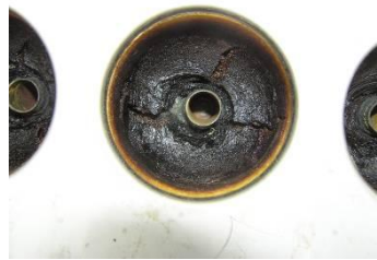
Figure 23 Degradation of PU foam insulation in manifold casing after exposure test
