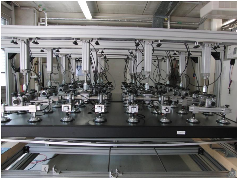
Figure 7. Mechanical load test at TUV using the manufacturers' original mounting equipment
