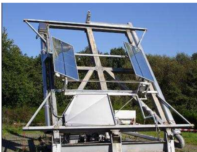
Figure 3: Testing of two PTC 1000 modular parabolic trough collectors at DLR in Germany.
