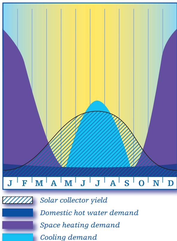
Solar thermal can cover a substantial part of the heating and cooling demand in a typical Central European building.
